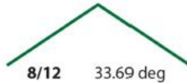
Examples: Diagrams showing minimum 4/12 and maximum 8/12 roof pitches.
