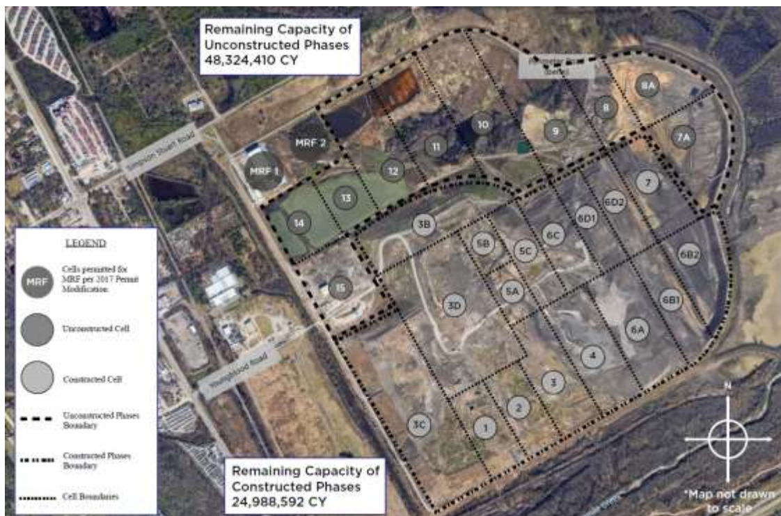
Figure E-1: Currently Constructed and Planned Landfill Cells
