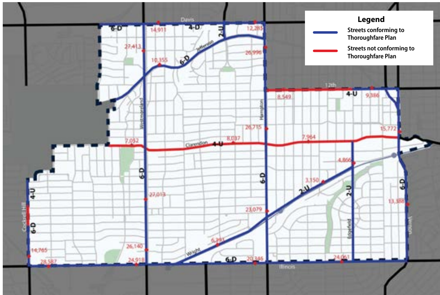
City of Dallas Thoroughfare Plan for West Oak Cliff with traffic counts added
