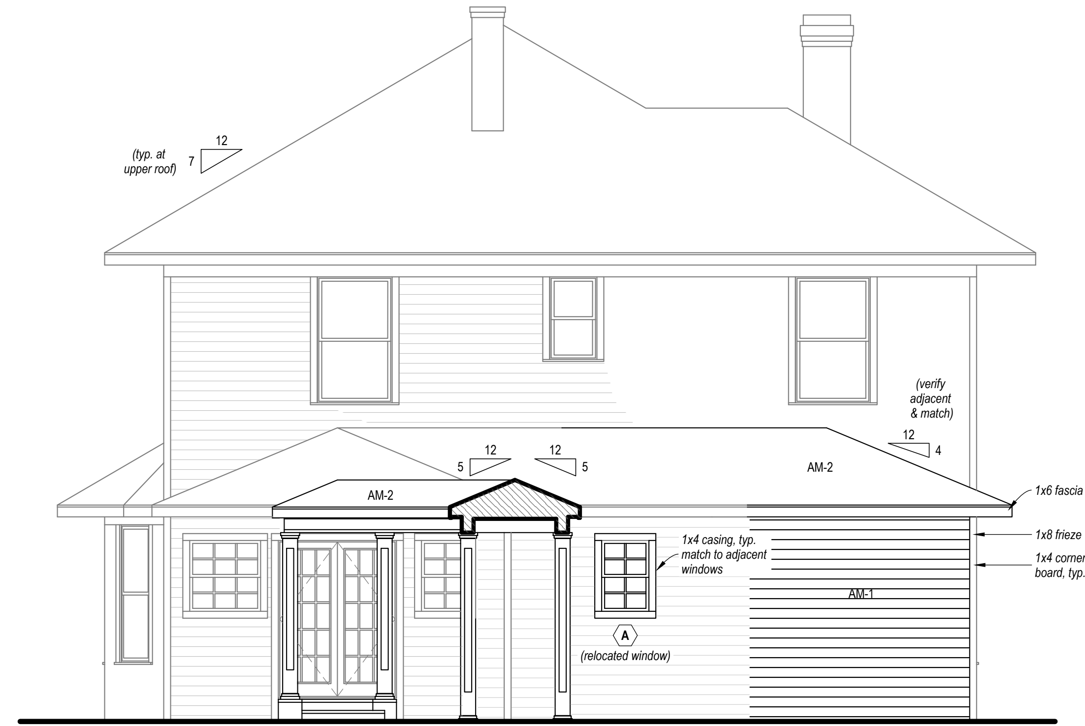
NORTH ELEVATION (HOUSE) scale: 1/4" = 1'-0"
