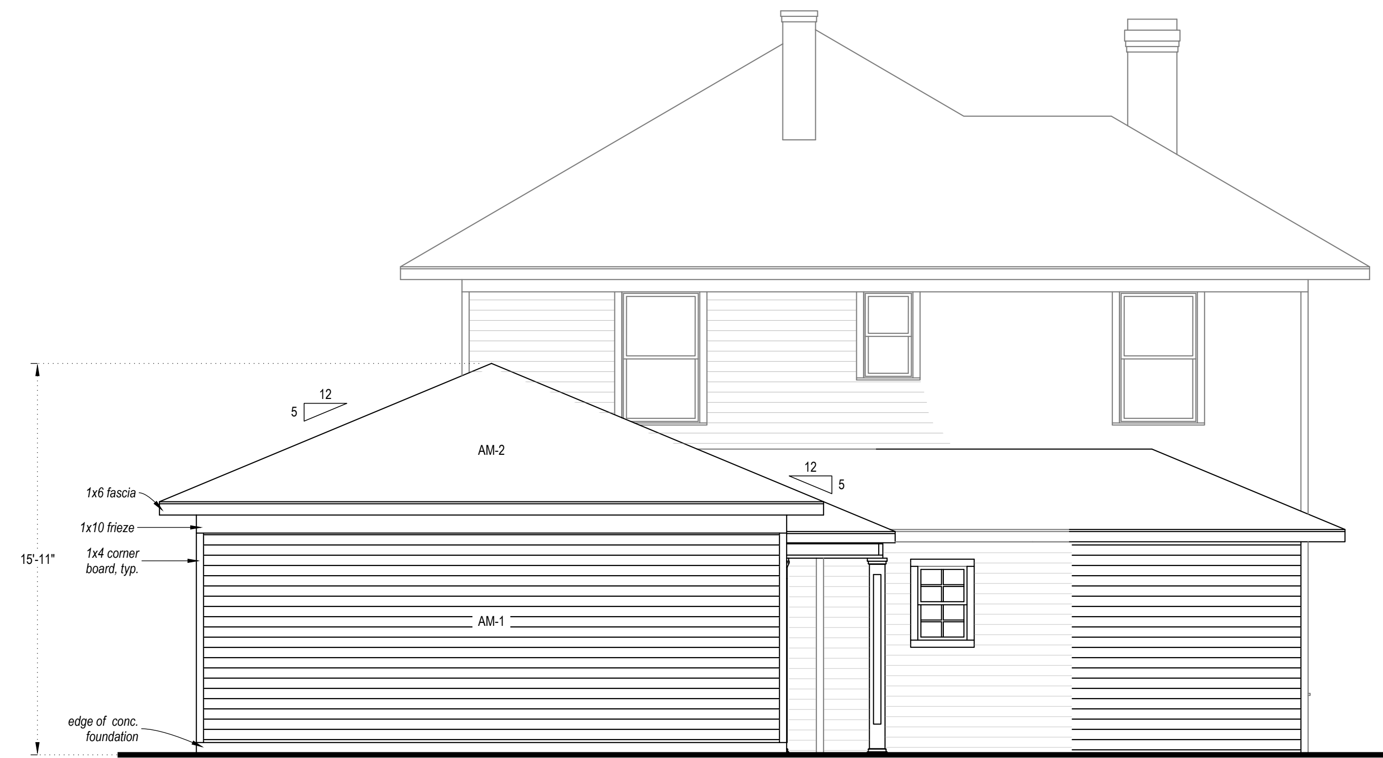
NORTH ELEVATION (GARAGE) scale: 1/4" = 1'-0"
