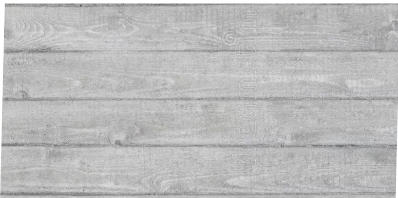
Concrete 1 Horizontal board formed
