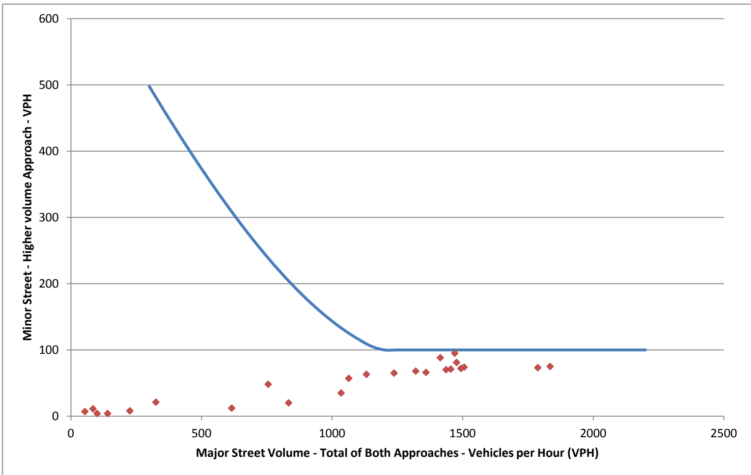
Figure 4C-4, Peak Hour Warrant, Major Street 2 lanes or more, Minor Street 2 lanes or more, Speed > 40 mph
