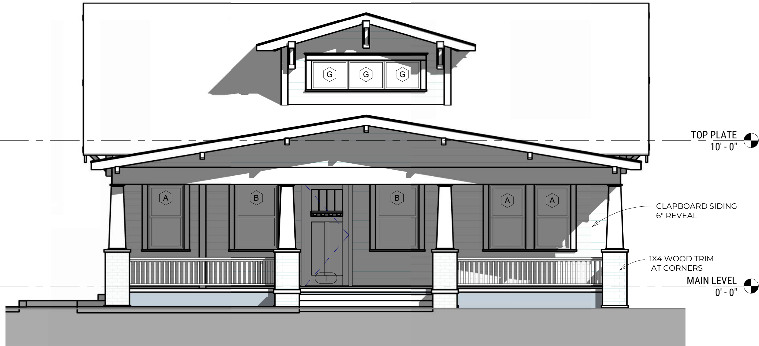
1 NORTHWEST ELEVATION (FRONT) 1/4" = 1'-0"
