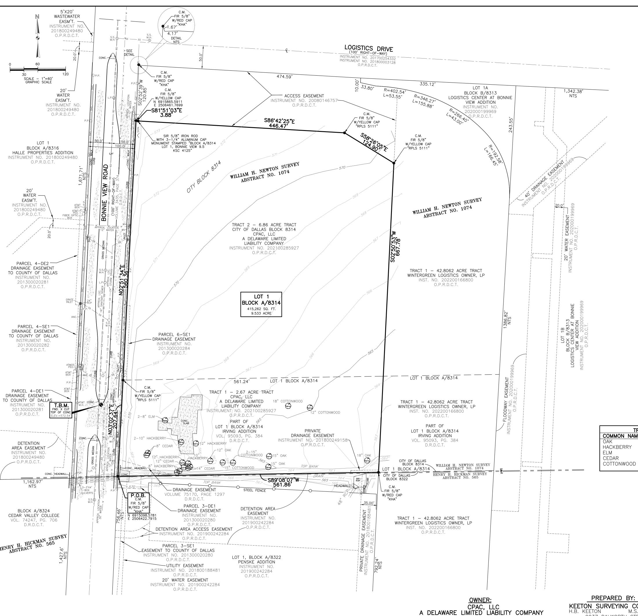
1. Basis of bearing is based on Grid North of the Texas State Plane Coordinate system, North Texas Central Zone 4202, North American Datum of 1983. Adjustment realization 2011.
