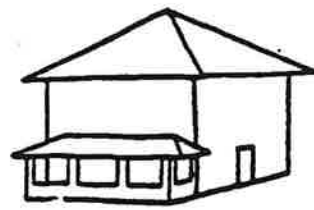
HIPPED ROOF, SYMMETRICAL, NO FRONT ENTRY
