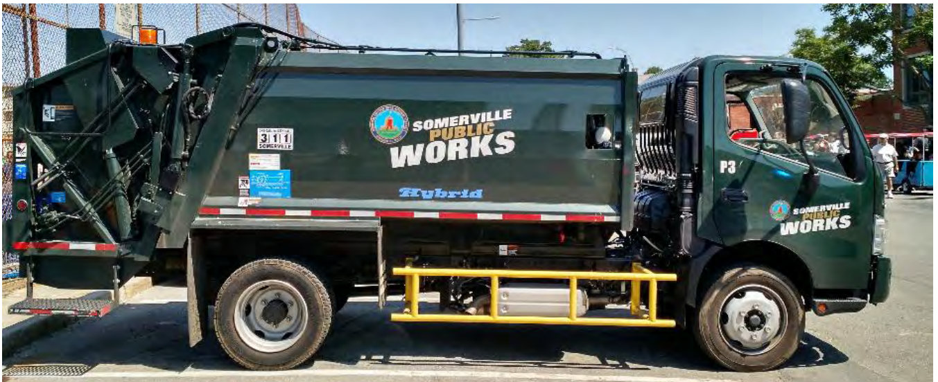
Figure 24: The compact Hino cab-over refuse truck used by Somerville (MA).
