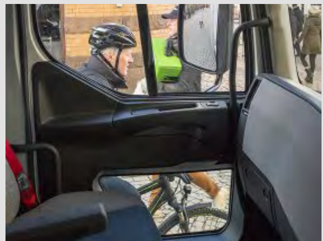
Figure 15 (top): The Mercedes Benz Econic MGT Euro5 high-vision cab in use for freight in Europe.
