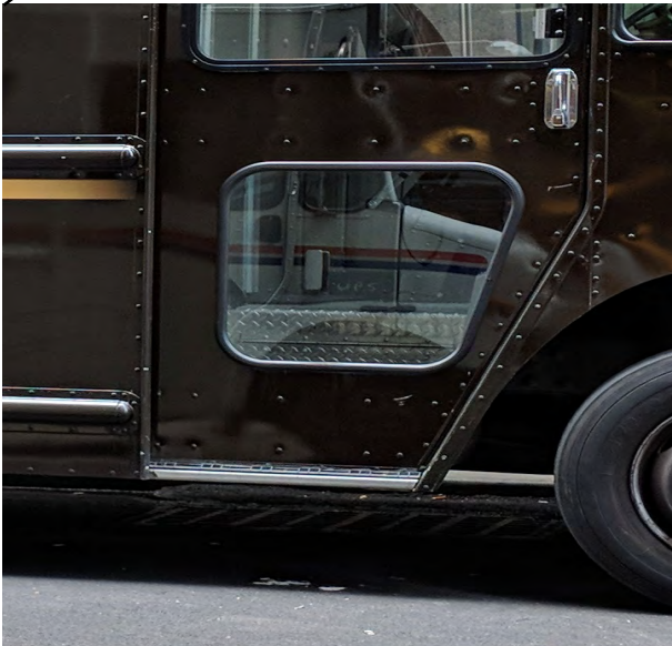
Figure 29: In-door peep windows on a UPS truck in New York City
