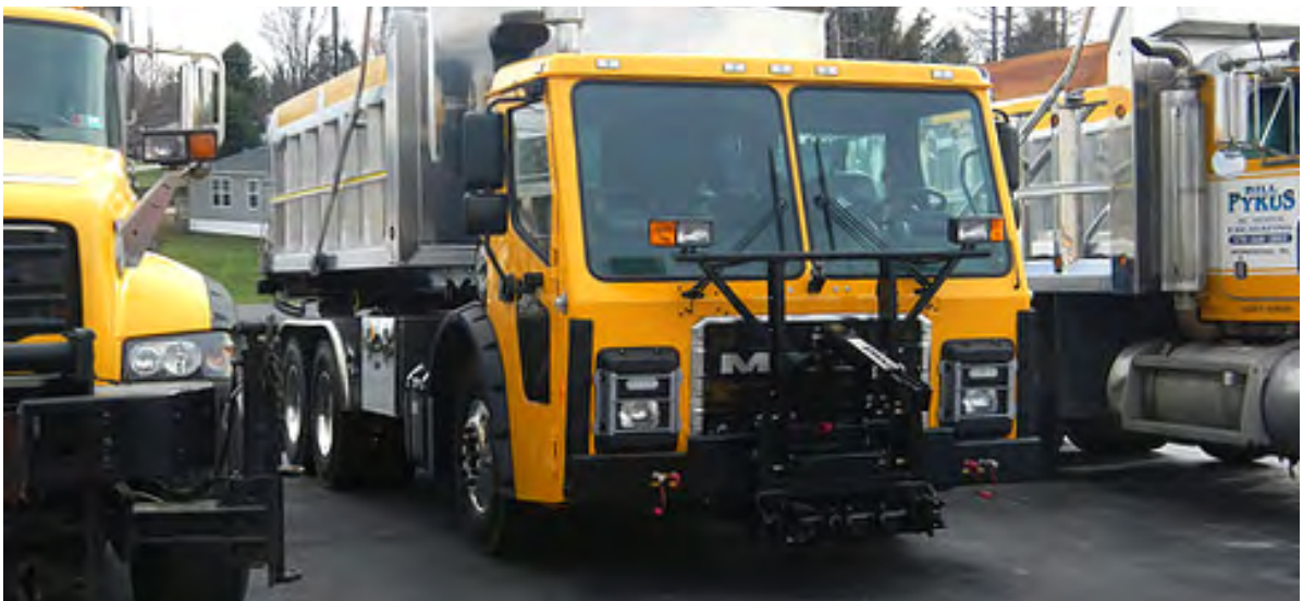
Figure 19: Progression from a low vision truck cab to a high-vision truck cab can be incremental or transformative. Image adapted by NACTO
