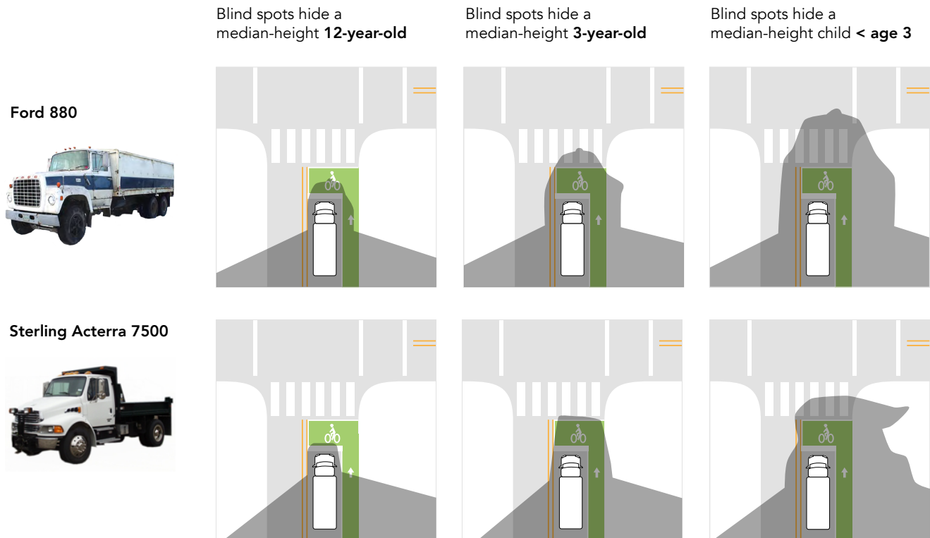
Figure 4: A vehicle with smaller blind spots better allows a median-height driver to see people in a bike box or a crosswalk, especially children. For the 50% of drivers who are below median height, the blind spots are actually larger than shown. 10
