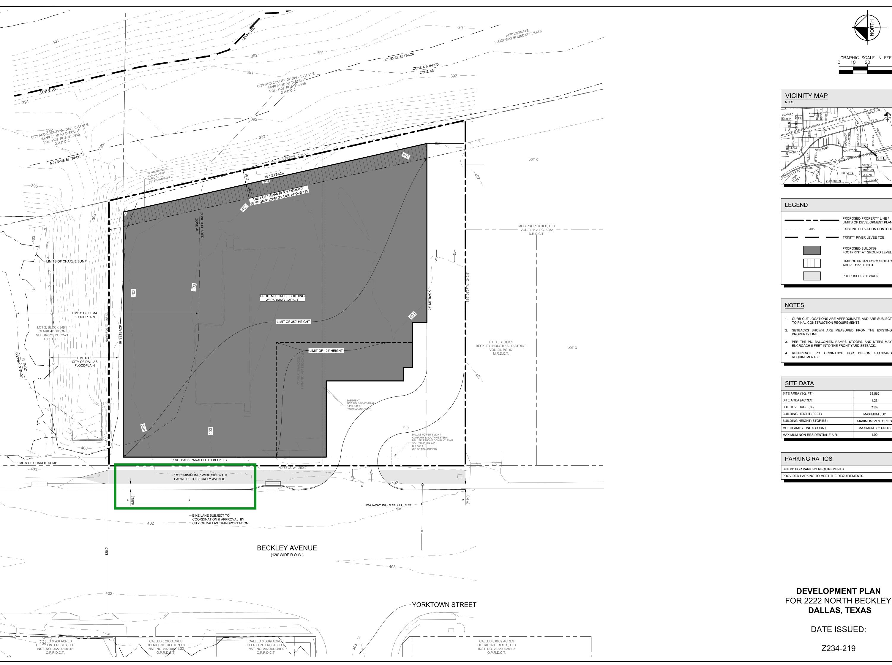
PROPOSED PROPERTY LINE / LIMITS OF DEVELOPMENT PLAN TRINITY RIVER LEVEE TOE PROPOSED BUILDING FOOTPRINT AT GROUND LEVEL LIMIT OF URBAN FORM SETBAC ABOVE 125' HEIGHT PROPOSED SIDEWALK
