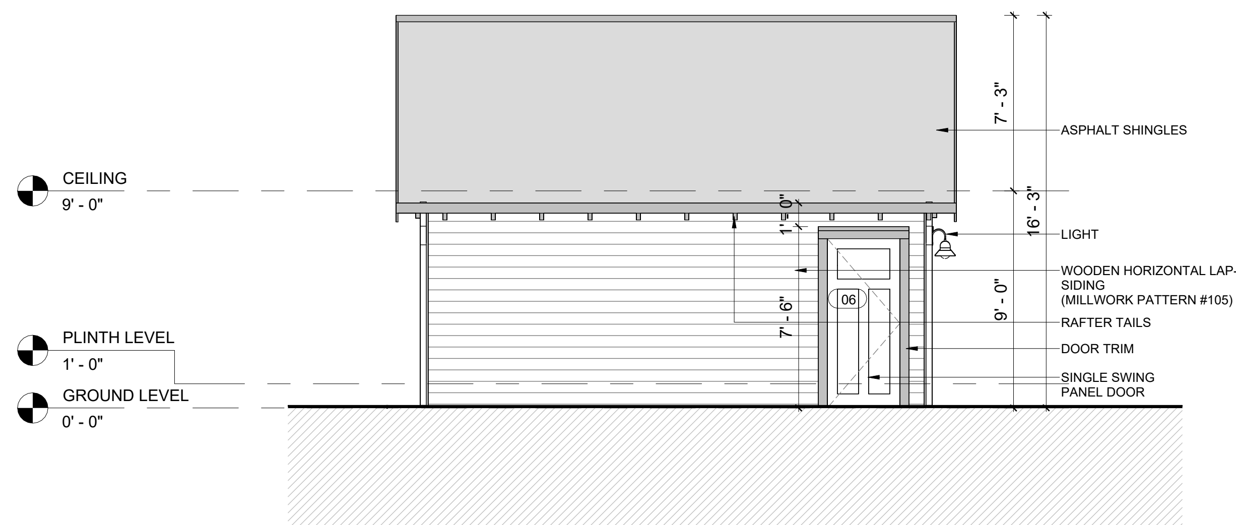
03 EAST SIDE ELEVATION-GARAGE 1/4" = 1'-0"
