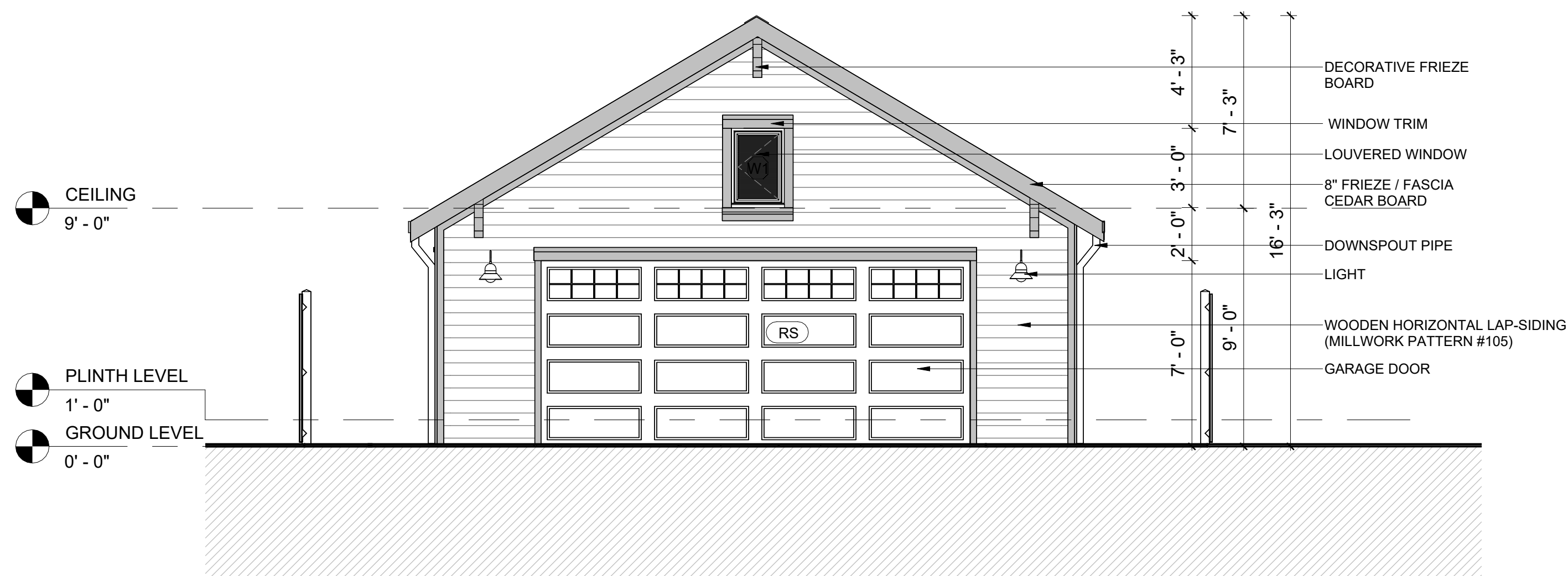
01 NORTH SIDE ELEVATION 1/4" = 1'-0"
