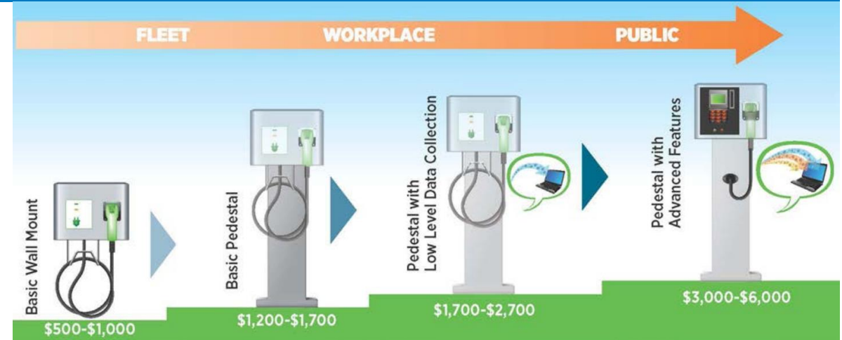
Figure 5. Ballpark cost ranges for different tiers of Level 2 EVSE units. Image from Kristina Rivenbark, New West Technologies.
