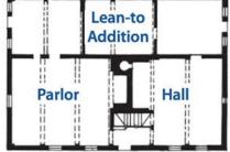
Figure 4. A typical New England saltbox features a steeply sloping roof to shed snow and a floor plan organized around a central chimney to conserve heat.
