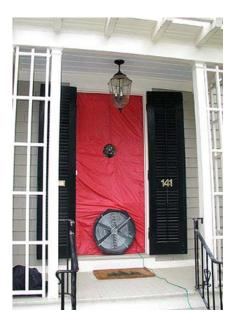
Figure 6. A blower door is used to depressurize a building by exhausting air at a rate that allows pressure gages and tracer smoke to measure the amount and location of air leakage. Photo: Robert Cagnetta, Heritage Restoration, Inc.
