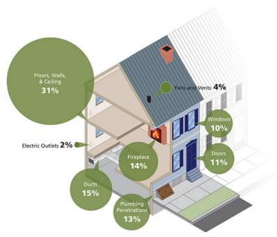
Figure 8. Where Air Escapes From a House (by percentage) – Image based on data from Energy Savers, U.S. Department of Energy. Illustration: Blank Space
