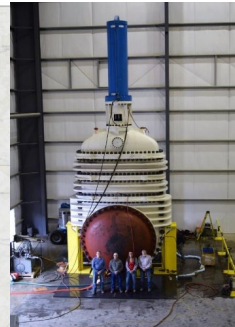
108-inch Gate Valve Installation
