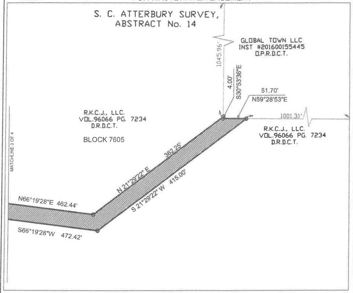
BASIS OF BEARING:Bearings are based on the Texas State Plane Coordinate System, North Central Zone 4202, North American Datum of 1983.
