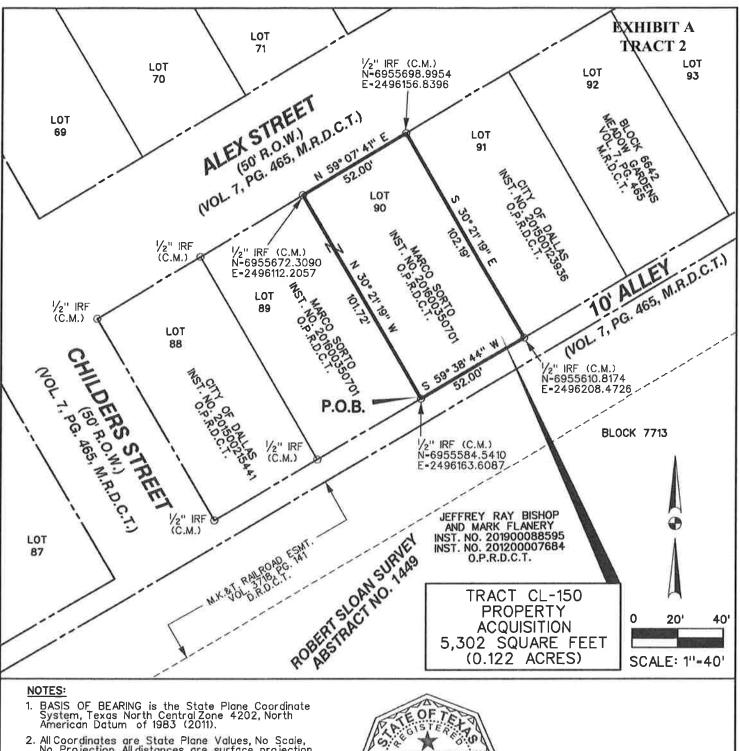
All Coordinates are State Plane Values, No Scale, No Projection. All distances are surface projection, using a scale factor of 1.000136506.
