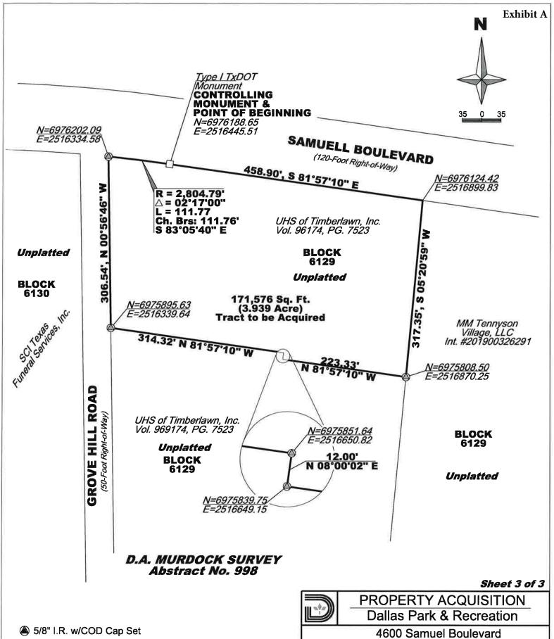
Basis of Bearings: Bearings are based on the State Plane Coordinate System, Texas North Central Zone 4202, North American Datum of 1983. All Coordinates shown are State Plane values No Scale, No Projection.
