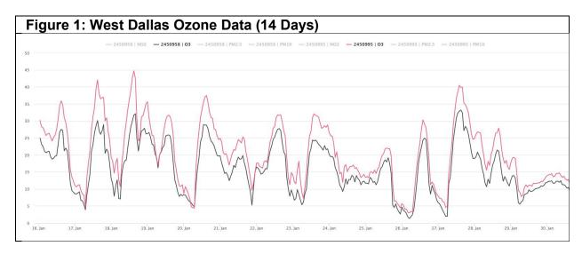
The ozone data in this example shows how close the two sensors in West Dallas are reading. There are some periods when the two sensors deviate, but overall the sensors are operating within the margin of error provided by the manufacturer. Figure 2 provides a similar comparison of the  $PM_{2.5}$  data for the two sensors.
