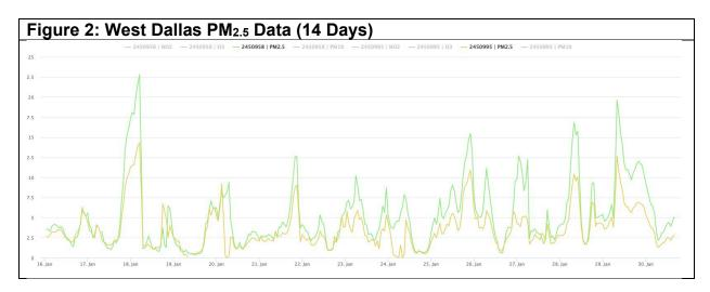
This  $PM_{2.5}$  data is similar to the ozone data, and the two sensors are reading consistently. This will provide more confidence in the detailed analysis that will be carried out on the data in the future.  $NO_2$  and  $PM_{10}$  data is consistent with these results. Overall, the sensors are performing as expected. Over time, more details will emerge from the data and allow more in-depth analysis.
