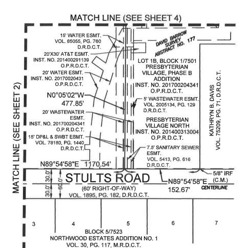
**LEGEND** P.O.B. = POINT OF BEGINNING  $\Delta$  = CENTRAL ANGLE IRF = IRON ROD FOUND IPF = IRON PIPE FOUND (C.M.) = CONTROLLING MONUMENT ESMT. = EASEMENT VOL. = VOLUME PG. = PAGE INST. NO. = INSTRUMENT NUMBER DP&L = DALLAS POWER & LIGHT SWBT = SOUTHWESTERN BELL TELEPHONE COMPANY D.R.D.C.T. = DEED RECORDS, DALLAS COUNTY, TEXAS O.P.R.D.C.T. = OFFICIAL PUBLIC RECORDS, DALLAS
