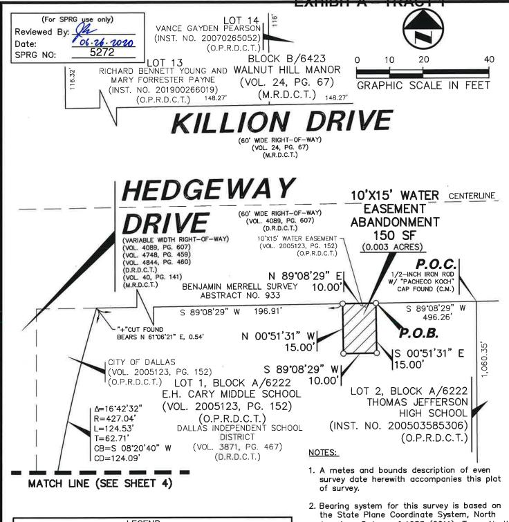
American Datum of 1983 (2011), Texas North Central Zone 4202. Distances shown hereon have been adjusted to surface by applying the Dallas County TxDOT combination factor of 1.000136506.
