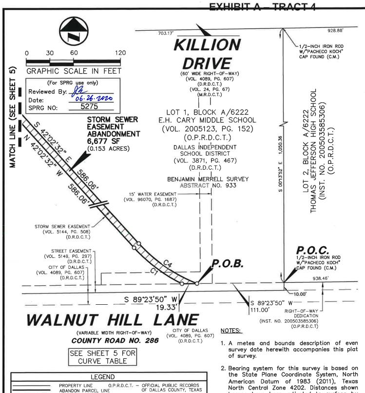
North Central Zone 4202. Distances shown hereon have been adjusted to surface by Dallas TxDOT the County combination factor of 1.000136506.
