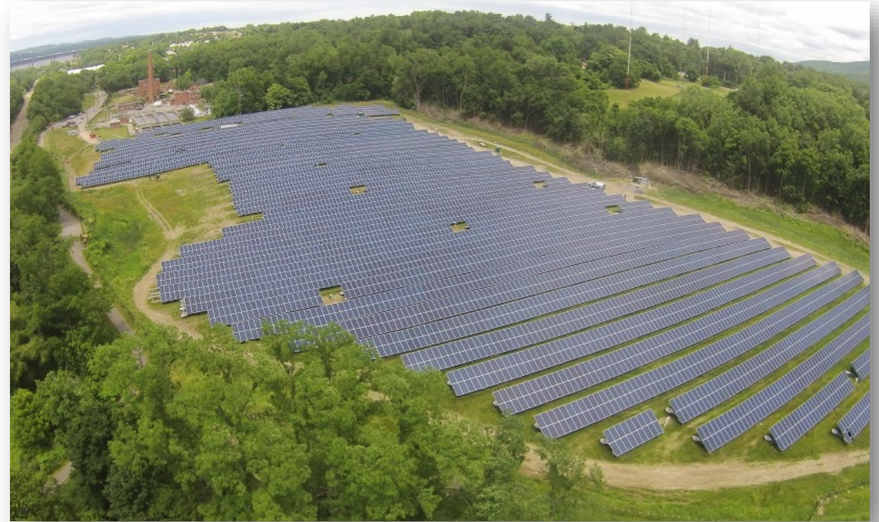
2 MW Solar Farm on a closed landfill in Beacon, NY (20 acres)
