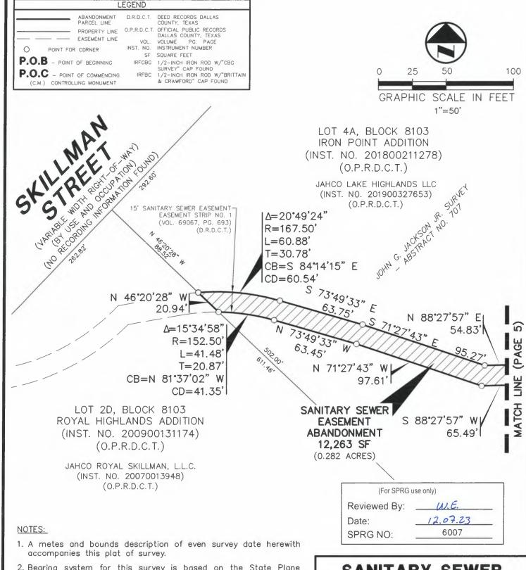
2. Bearing system for this survey is based on the State Plane Coordinate System, North American Datum of 1983 (2011), Texas North Central Zone 4202. Distances reported have been scaled by applying the Dallas County TxDOT surface adjustment factor of 1.000136506.
