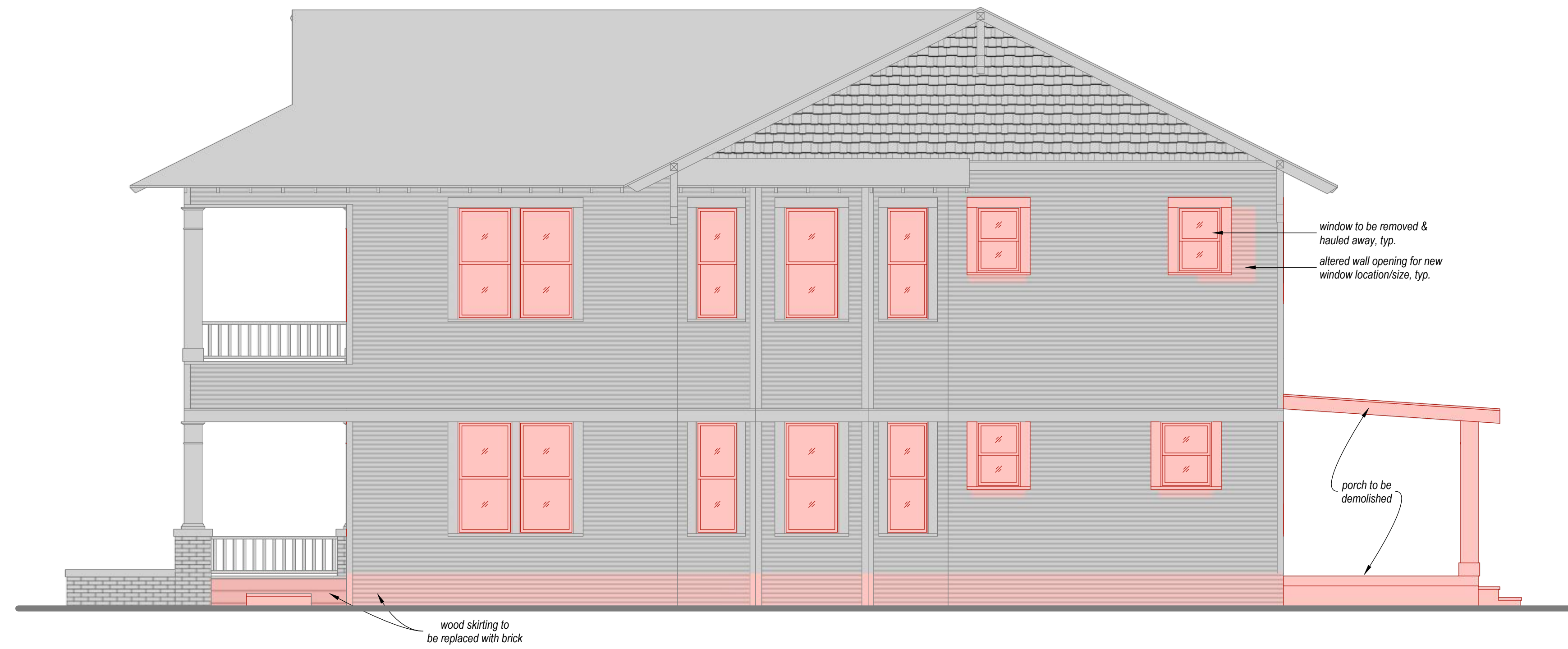
DEMOLITION ELEVATION (RIGHT SIDE)
