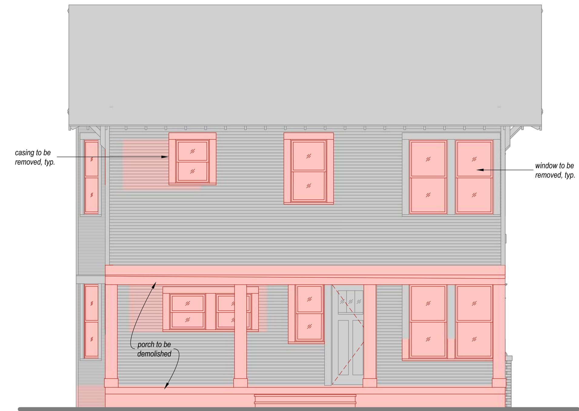
DEMOLITION ELEVATION (REAR)
