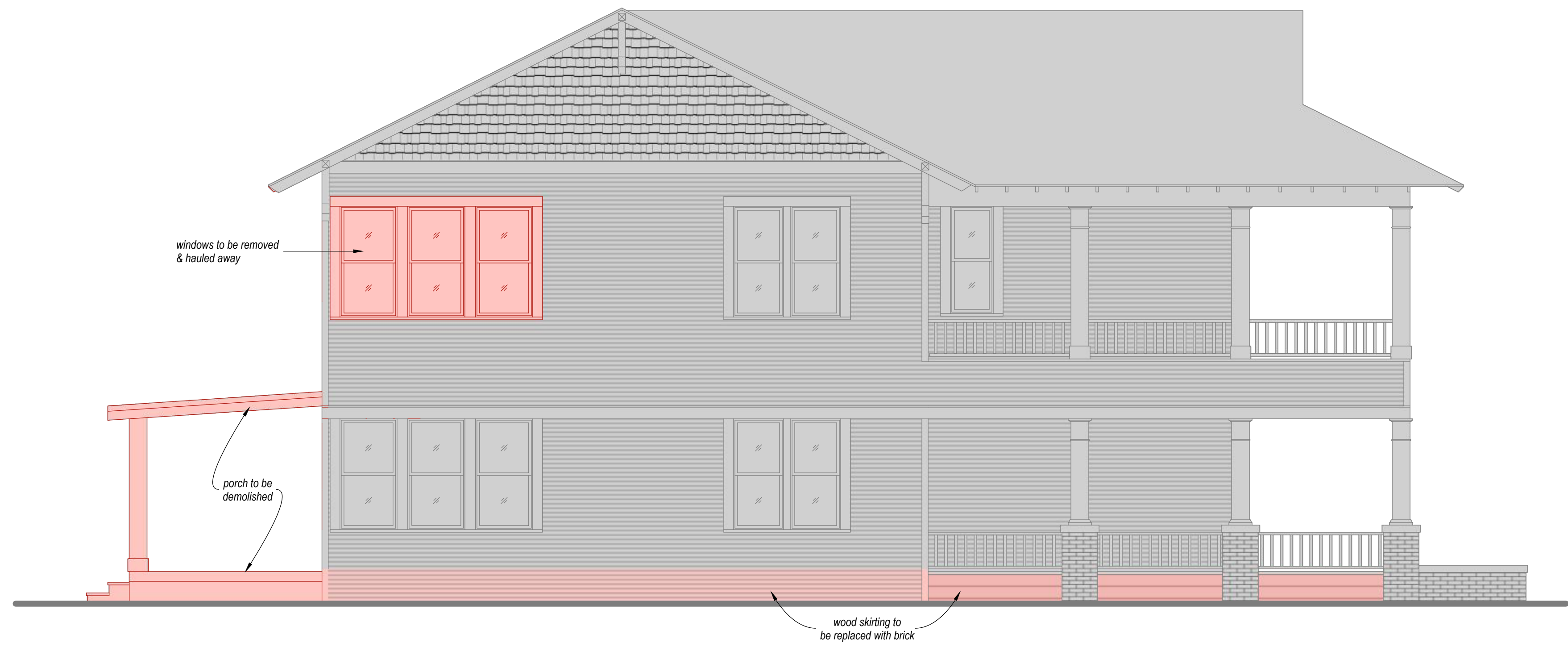
DEMOLITION ELEVATION (LEFT SIDE)
