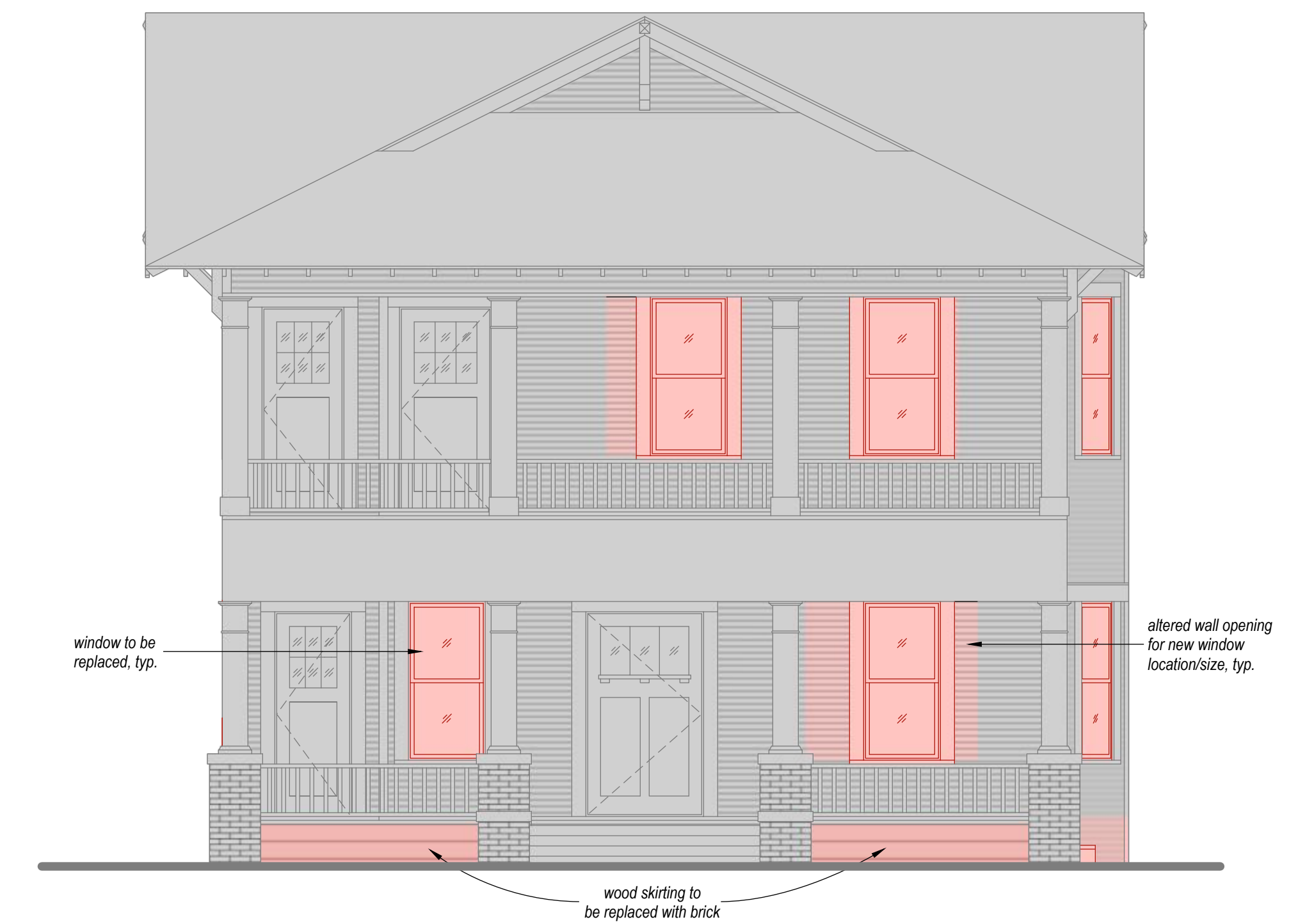
DEMOLITION ELEVATION (FRONT)
