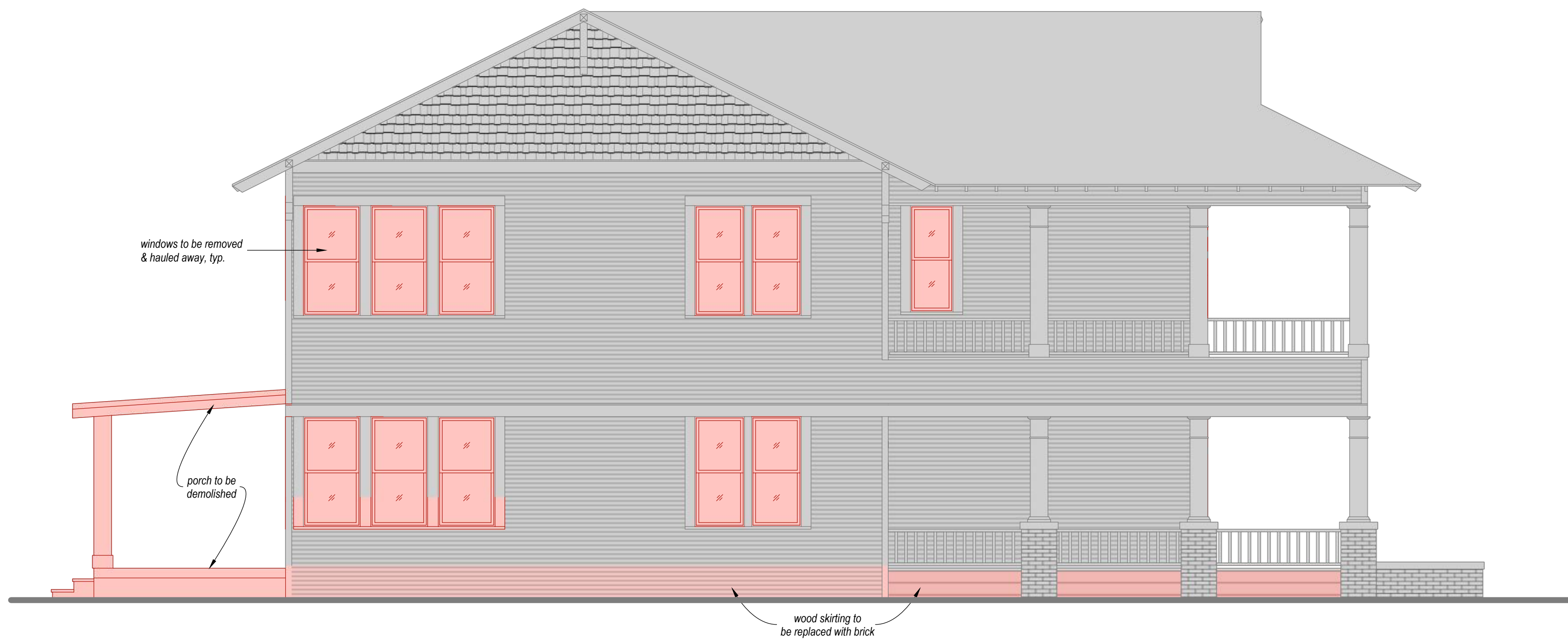
DEMOLITION ELEVATION (LEFT SIDE)
